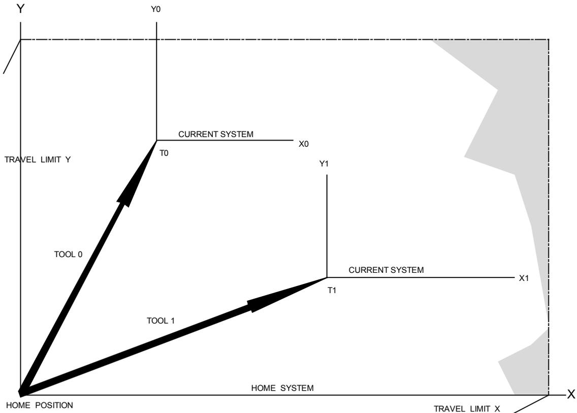
**Figure 3-2 : The UNIPROG Coordinate System**
