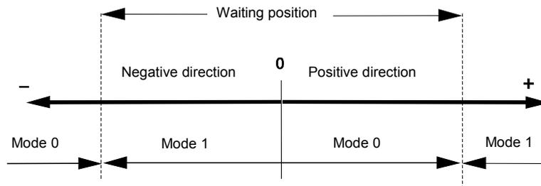
**Figure 8-4 : Waiting position according to the displacement direction**
